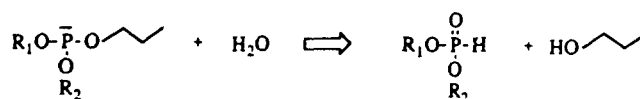
Scheme 6 Phosphite sensitivity to hydrolysis and subsequent molecular weight decrease ( R_1 and R_2 = phenyl groups or polyester chains)
